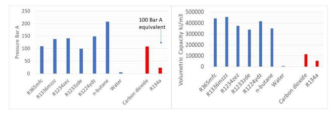
Figure 8: Pressure at 230 deg. C and Volumetric Capacity for Gas Cooler Sizing
