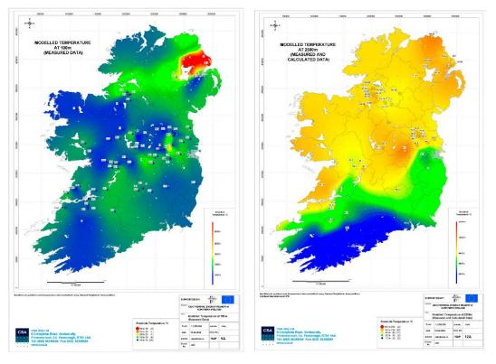
Figure 1: Modelled Temperature at 100m and 2500m based on Measured Data (Kelly et al, 2005)
