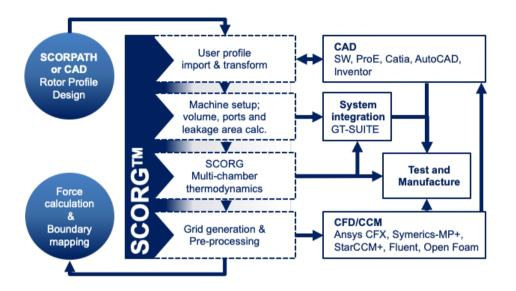
SCORG<sup>™</sup> is industry leading software for design and analysis of screw compressors, expanders, pumps and motors
