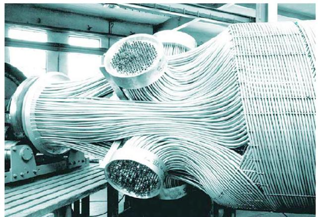
Fig. 10. Tube to tube sheet connection areas on a coil wound heat exchanger (Roos et al. [42]).
