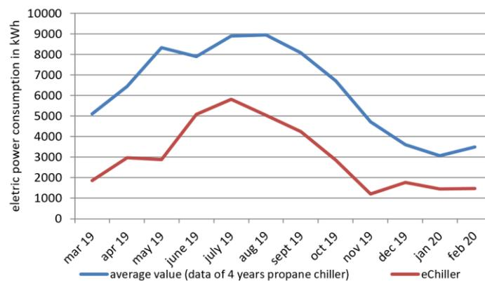
**Figure 6. Comparison of performance R718 (eChiller) vs R290**
