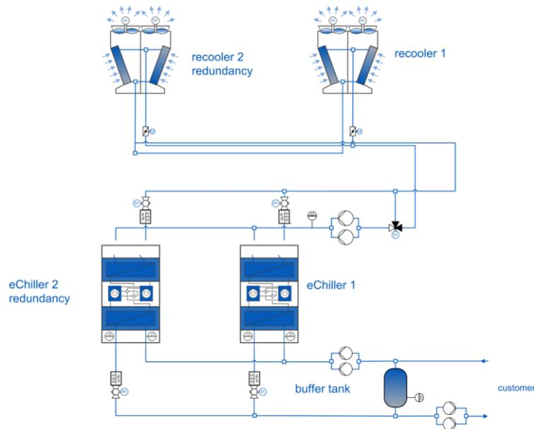
**Figure 2. Typical n+1 R718 Chiller configuration**
