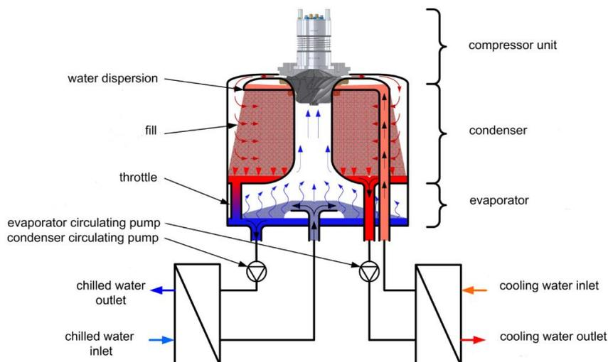
**Figure 5. External Heat Exchanger system**
