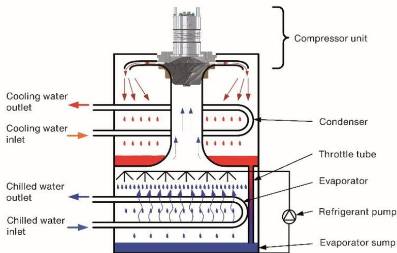
**Figure 4. Internal Heat Exchanger system**
