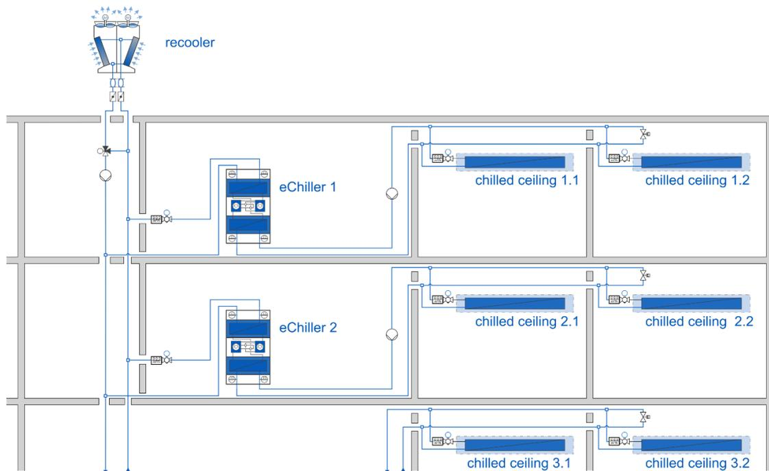
**Figure 1. Central Adiabatic Cooler supplying 2 x internally located R718 Chiller units (eChiller)**
