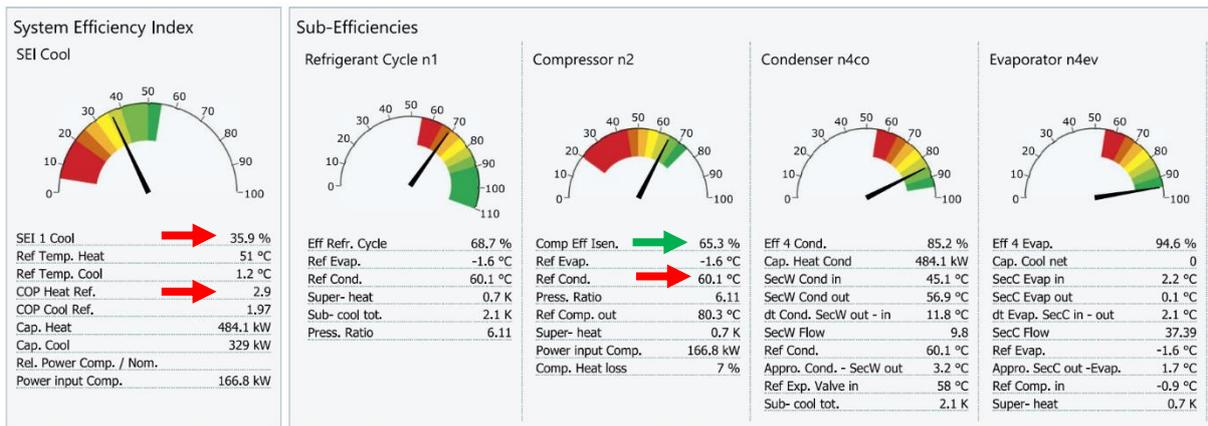
Figure 3. Ground source heat pump operating with full capacity at high temperatures in heating system reaching a COP heating of 2.9
