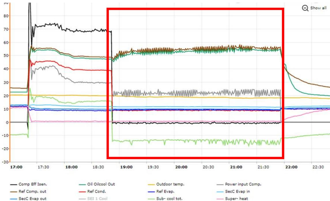
**Figure 10. Chiller is in the red box operating 3 hours without pressure increase due to the mechanism for unloaded start being activated. During this time no cooling capacity is generated and there is significant risk for damage**
