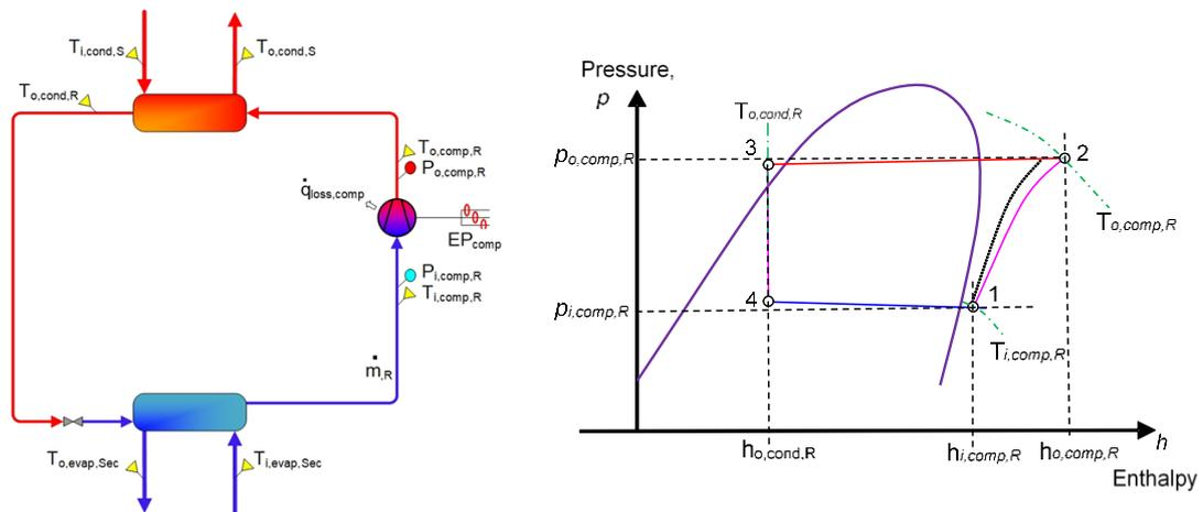
**Figure 1. Sensor required to analyse capacity and performance of a refrigeration process and the points defined in a pressure enthalpy graph**
