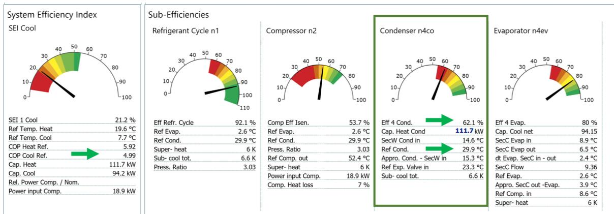
**Figure 7. Performance of the air-cooled chiller after adjusted fan control efficiency has increased with 30%**
