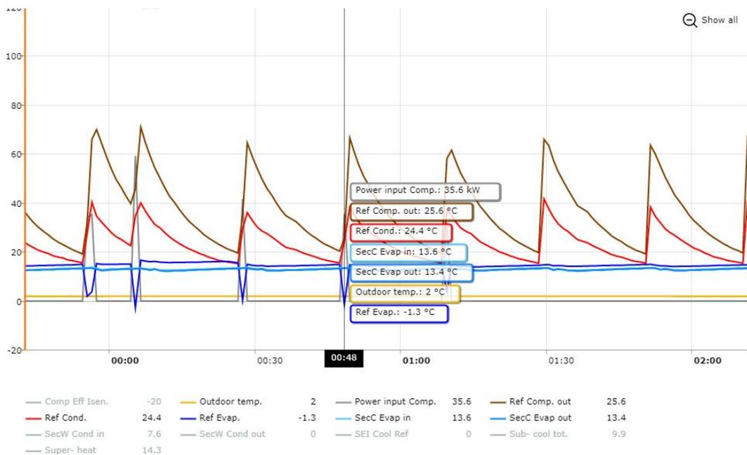
**Figure 9. Example of chiller running on ten minutes restart protection**
