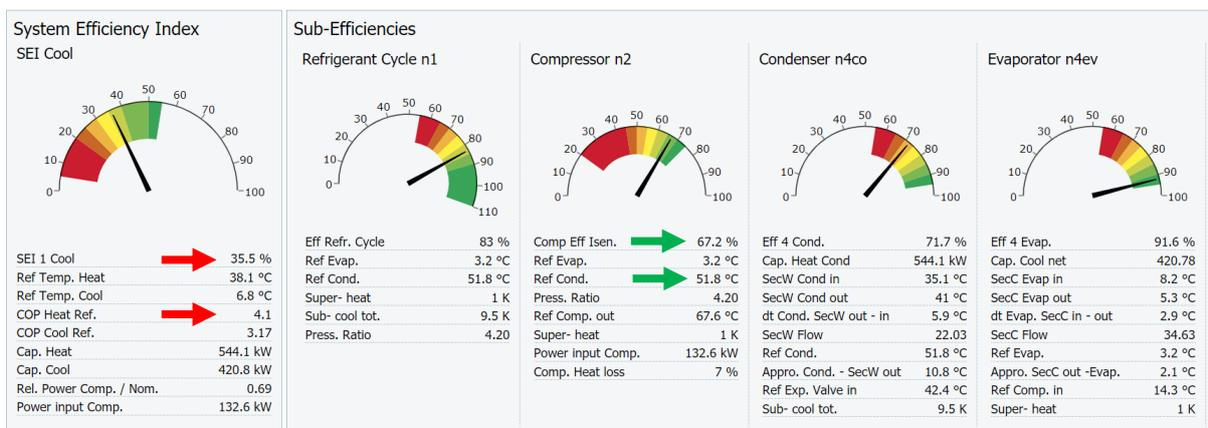
Figure 4. Same heat pump at lower temperatures in heating system reaching COP of 4.1 this is 41% better COP than operating conditions above but system is as efficient (35%) as shown by the SEI
