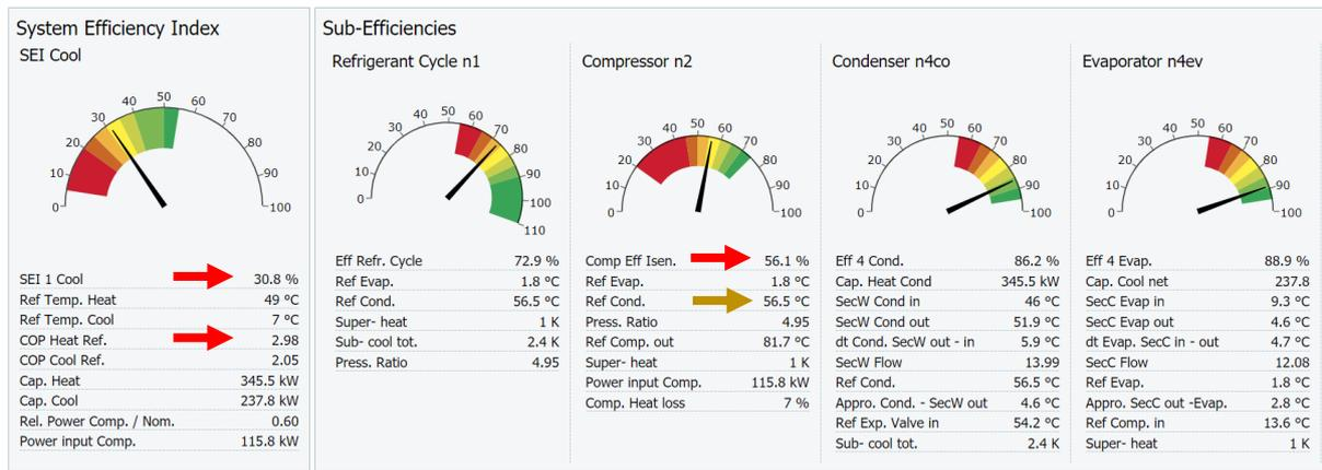
**Figure 5. Same heat pump at part load - reducing screw compressor efficiency to reduce COP heat to 2.98 the reduction of compressor efficiency also has a direct impact on SEI that is reduced to 30.8%**
