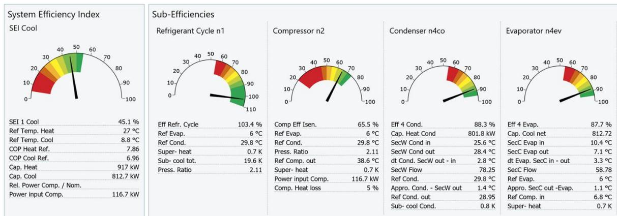
**Figure 2. A high efficiency chiller with COP 6.96 this is operating with economiser offering a high cycle efficiency**
