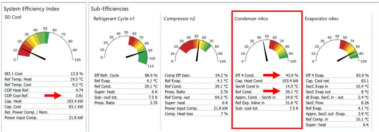
**Figure 6. Air-cooled chiller operating at low ambient conditions condensing at 39°C due to default setting of fan controller**
