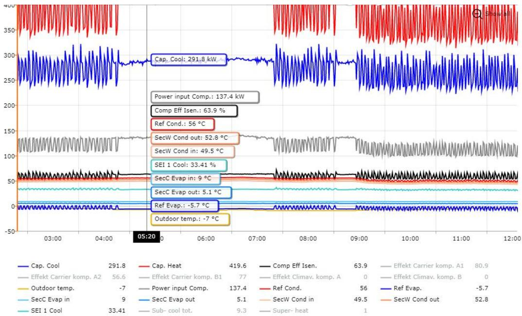
**Figure 8. Capacity control that is unstable during a majority of the time of operation shown – Grey is power, blue cooling capacity and red heating capacity**
