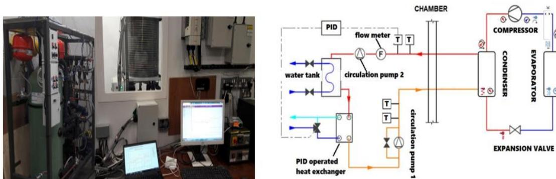
Figure 2: Heat Pump Test Facility
