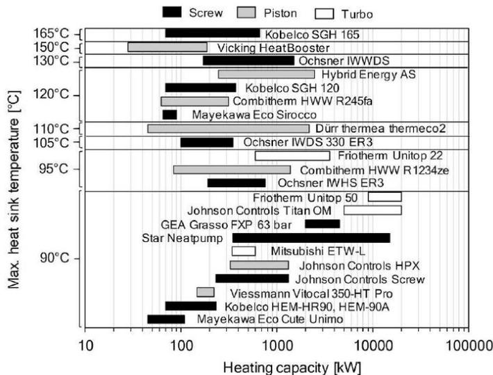
Figure 6: Heat Pump Types
