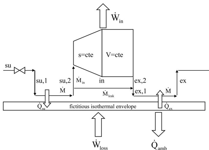
Figure 5: Semi empirical scroll expander model (adapted from Lemort et al, 2009)
