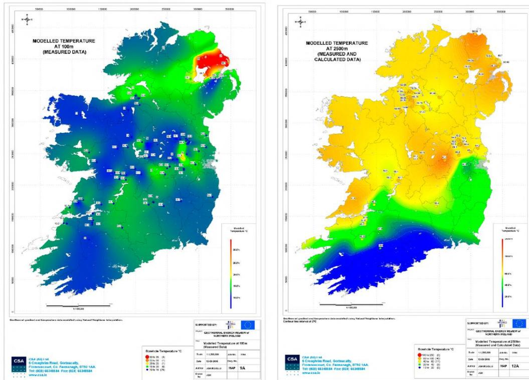
Figure 1: Modelled Temperature at 100m and 2500m based on Measured Data (Kelly et al, 2005)
