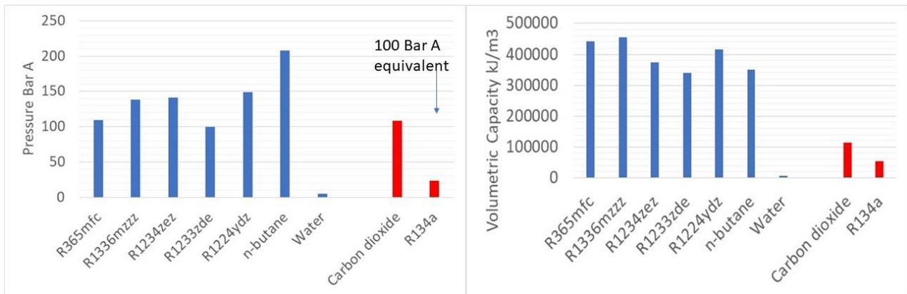
Figure 8: Pressure at 230 deg. C and Volumetric Capacity for Gas Cooler Sizing
