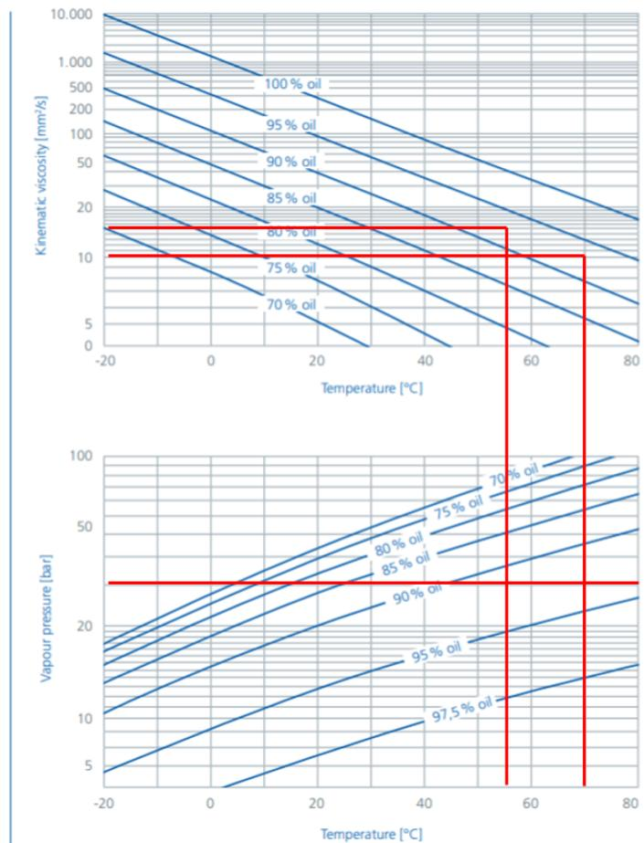
**Figure 3. @30/100 bar the viscosity of the oil is double with the external discharge manifold**
