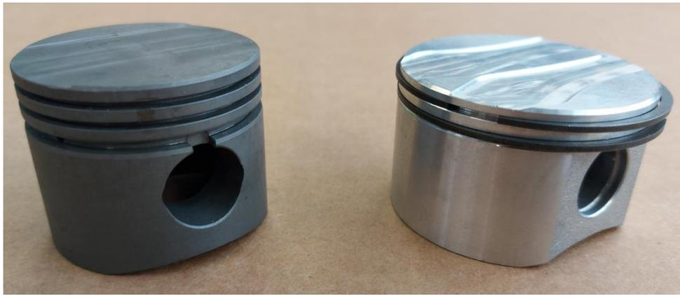
**Figure 6. Cast iron pistons have about double the surface HB hardness of the Aluminium ones and expand Half due to the thermal expansion. Photo: Dorin property**
