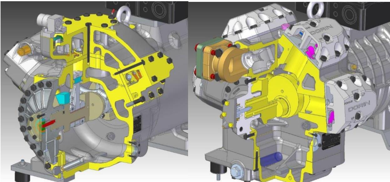
Figure 5. Benefits of the external manifold (left) compared to a standard design (right). Dorin property
