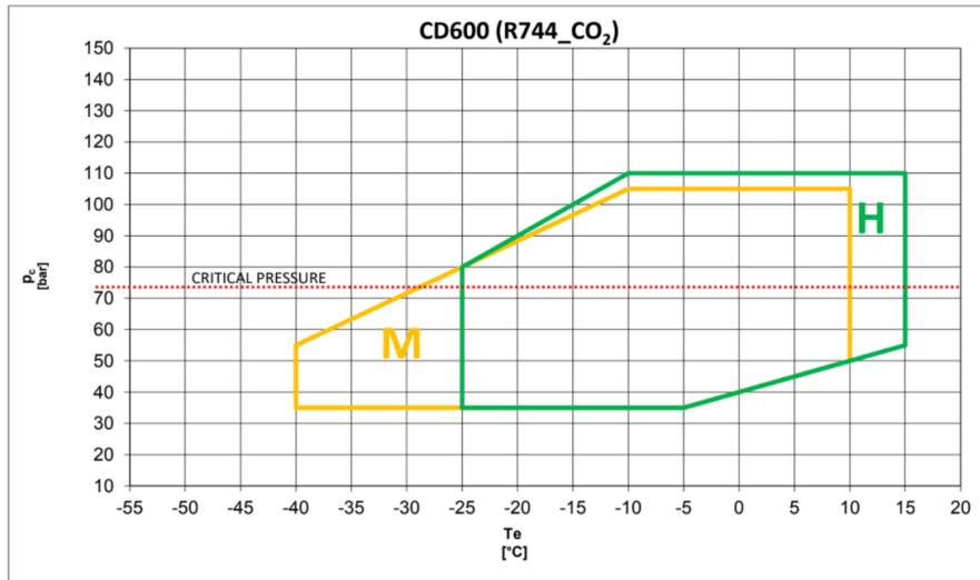
Figure 4. The application envelope from Dorin Selection Software
