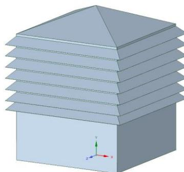
**Figure 2. CAD representation of the wind tower and heat pipe arrangement.**
