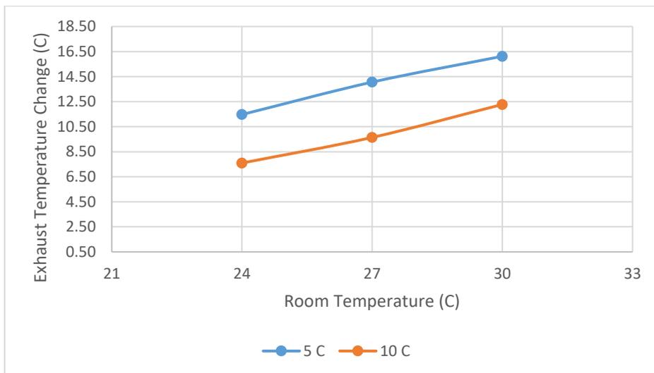
**Figure 10. Exhaust temperature change for 2 ms<sup>-1</sup> wind speed**
