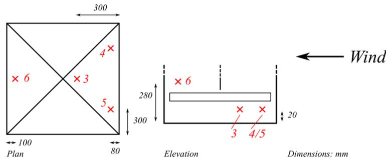
Figure 7. Location of the wind tower internal measuring points
