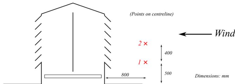
Figure 6. Location of the external measuring points
