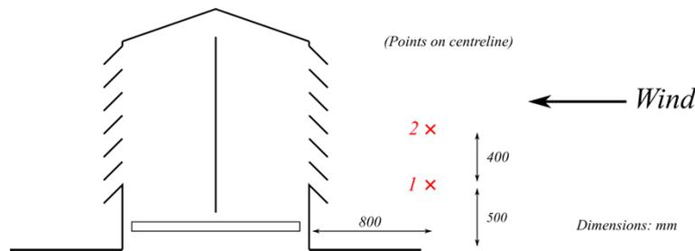
Figure 6. Location of the external measuring points
