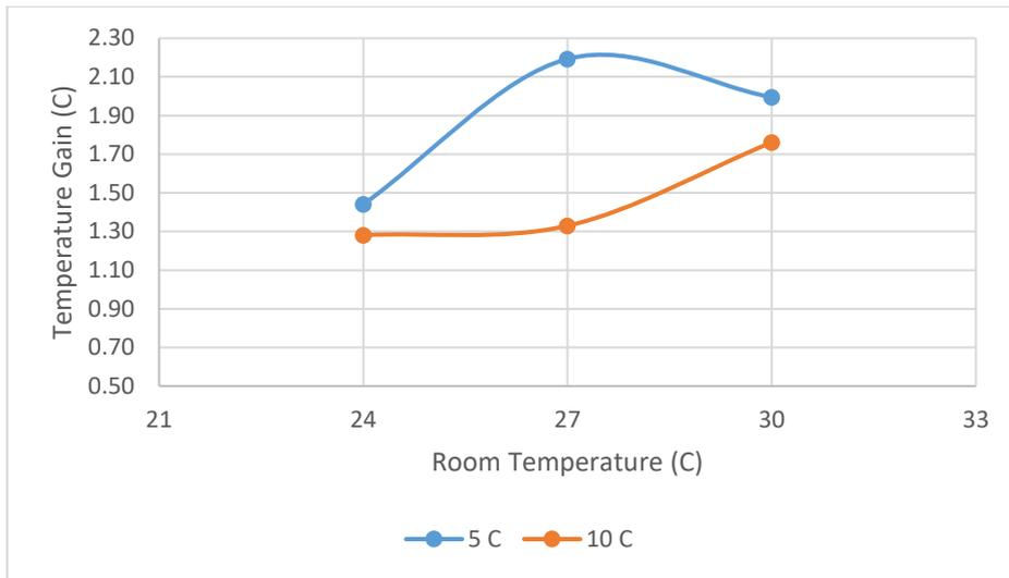
**Figure 8. Temperature gain to the incoming air for 2 ms<sup>-1</sup> wind speed**
