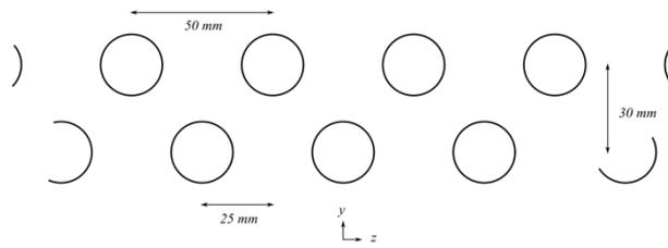
**Figure 3. Heat pipe arrangement**
