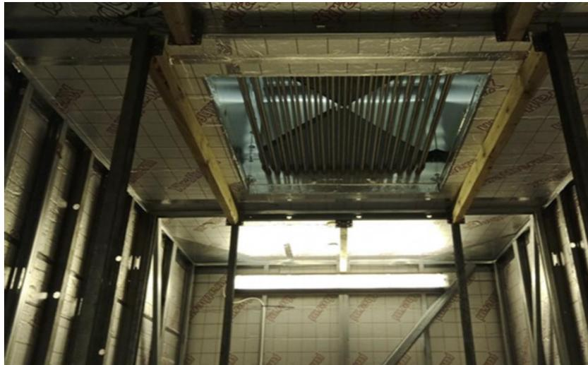
**Figure 4. Wind tower and heat pipes viewed from within the test room**
