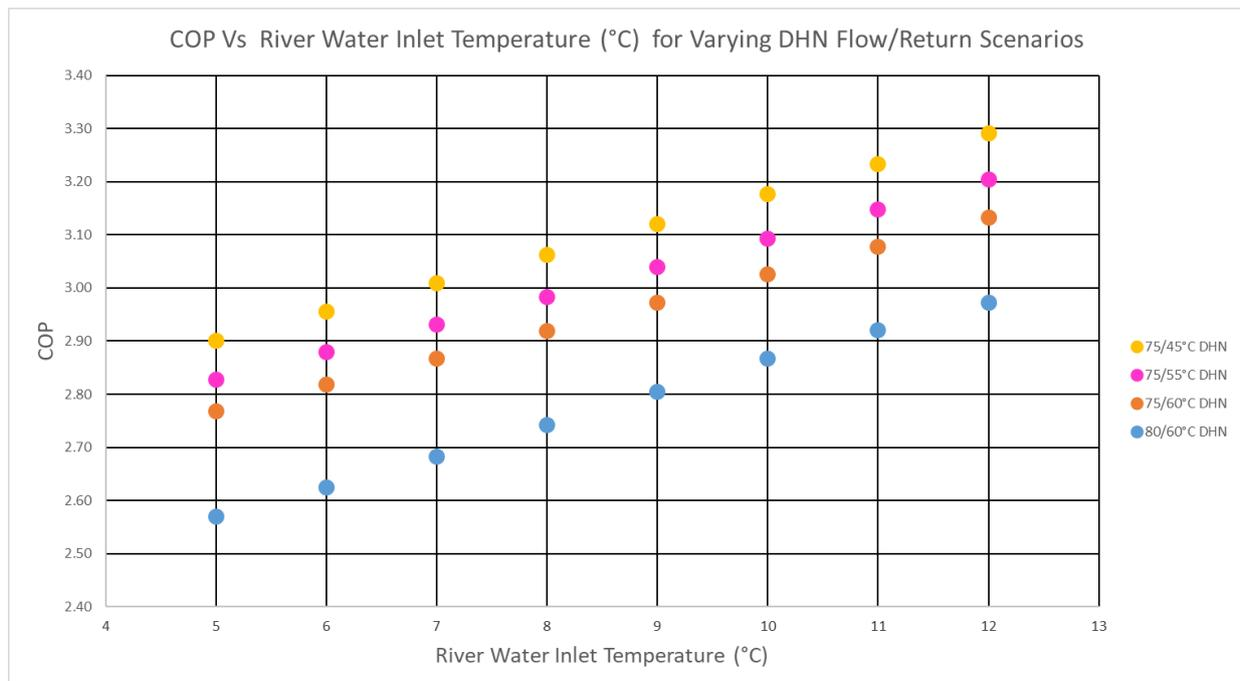
**Figure 4 – Calculated COP for the district loop under different conditions**
