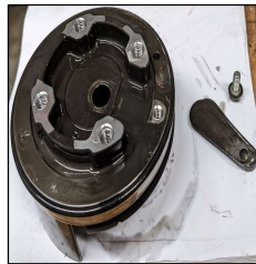
Discharge side with the check valve removed
