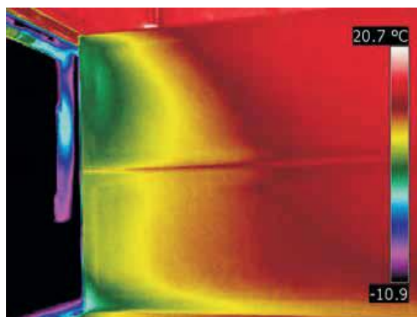
Figure. 3 Air separation in operation at open cold store doorway
