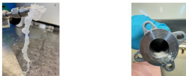
Figure 4: Discharged polymerised HFO-1234yf (originating as R-513A) (Ignatowicz et al., 2026)
