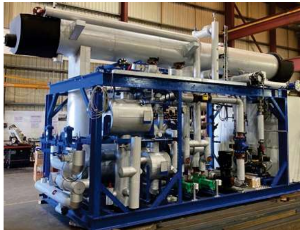
Figure 2: Packaged industrial heat pump in manufacture
